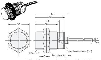
\* 6-dia. vinyl-insulated round cable with 3 conductors (Conductor cross section: 0.5 mm², Insulator diameter: 1.9 mm), Standard length: 2 m
