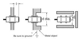
\* Be sure to ground the metal object, otherwise Sensor operation will not be
