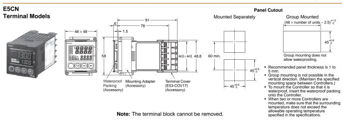
E5CN-U **Panel Cutout Plug-in Models** (84.7)Mounted Separately **Group Mounted** 14.2 2.5)+1.0 48 × 48 70.5 (48 × number of units 45<sup>+0.6</sup> 60 min · Recommended panel thickness is 1 to 5 mm.
