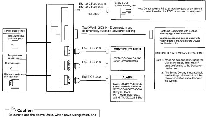
connection cables for the prevention of malfunctions or accidents that may be caused by mistakes in wiring. OMRON
