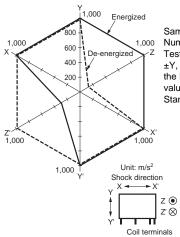
Sample: G6DN-1A Number of Relays: 5 pcs Test conditions: Impose a shock in the  $\pm X$ ,  $\pm Y$ , and  $\pm Z$  directions three times each with the Relay energized to check the shock values that cause the Relay to malfunction. Standard:100 m/s<sup>2</sup>
