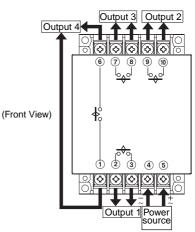
Note: 1. The Time Switch output uses a no-voltage contact. An external power supply is required for applications in which a load is driven.2. The output contact ratings are different for 2-circuit and 4-circuit models.
