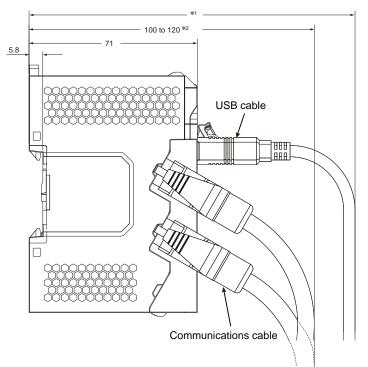
\*1. This dimension depends on the specifications of the commercially available USB cable. Check the specifications of the USB cable that is used. \*2. This is the dimension from the back of the Unit to the communications cables.
