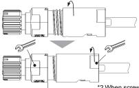
\*2 When screwing up the cap by large size tool, it may cause damage.
