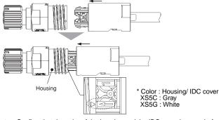
Note: Confirm that the color of the housing and the IDC cover is same before insertion.
