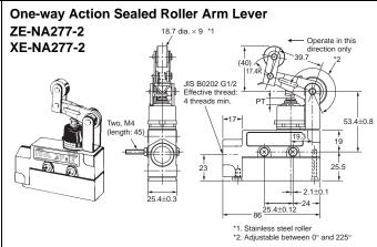
Note: 1. Unless otherwise specified, a tolerance of  $\pm 0.4$  mm applies to all dimensions.
