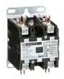
Contactor, Definite Purpose, 25A, 2 pole, 5 HP at 230 VAC, 1 phase, 208/240 VAC 60 Hz 220 VAC 50 Hz coil, open
