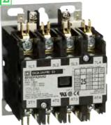
Contactor, Definite Purpose, 25A, 4 pole, 20 HP at 575 VAC, 3 phase, 110/120 VAC 50/60 Hz coil, open
