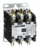
Contactor, Definite Purpose, 30A, 3 pole, 20 HP at 575 VAC, 3 phase, 208/240 VAC 60 Hz 220 VAC 50 Hz coil, open
