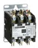
Contactor, Definite Purpose, 30A, 3 pole, 20 HP at 575 VAC, 3 phase, 24/24 VAC 50/60 Hz coil, open
