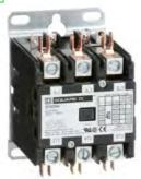
Contactor, Definite Purpose, 40A, 3 pole, 25 HP at 575 VAC, 3 phase, 440/480 VAC 50/60 Hz coil, open
