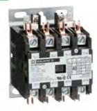
Contactor, Definite Purpose, 40A, 4 pole, 25 HP at 575 VAC, 3 phase, 110/120 VAC 50/60 Hz coil, open
