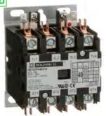
Contactor, Definite Purpose, 40A, 4 pole, 25 HP at 575 VAC, 3 phase, 24/24 VAC 50/60 Hz coil, open
