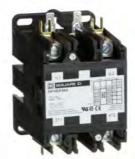
Contactor, Definite Purpose, 60A, 2 pole, 10 HP at 230 VAC, 1 phase, 110/120 VAC 50/60 Hz coil, open
