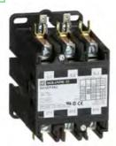
Contactor, Definite Purpose, 60A, 3 pole, 30 HP at 575 VAC, 3 phase, 110/120 VAC 50/60 Hz coil, open
