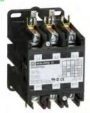
Contactor, Definite Purpose, 60A, 3 pole, 30 HP at 575 VAC, 3 phase, 24/24 VAC 50/60 Hz coil, open
