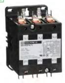
Contactor, Definite Purpose, 75A, 3 pole, 40 HP at 575 VAC, 3 phase, 110/120 VAC 50/60 Hz coil, open
