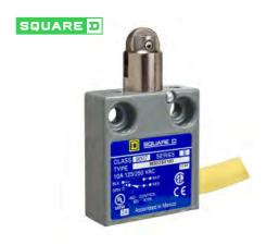
Limit switch, 9007MS, miniature, parallel roller plunger, 10A at 240VAC, 1NO/1NC, 6 feet of cable, side, NEMA 4, 6P, 13
