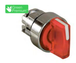
Harmony XB4, Illuminated selector switch head, metal, red, Ø22, integral LED, 3 positions, stay put
