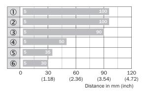
Max. sensing range S<sub>n</sub>, flush or non-flush installation, non-magnetizable material
