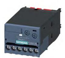
Electronic timing relay ON delay with semiconductor output 24-240 V AC/DC Time range 0.05...100 s can be snapped on at the front for contactors 3RT2 S00/S0 and auxiliary contactor 3RH2 S00 Screw terminal Varistor for attenuation of the contactor coils integrated
