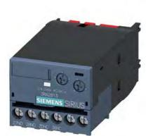
Solid-state time-delayed auxiliary switch ON delay Relay 1 NC + 1 NO 24...240 V AC/DC Time range 0.05...100 s Can be snapped on at the front For 3RT2 S00-S3 contactors and 3RH2 S00 contactor relays Screw terminal Varistor for attenuation of the contactor coils integrated
