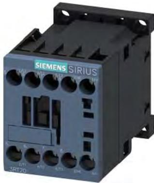
Power contactor, AC-3 16 A, 7.5 kW / 400 V 1 NC, 24 V DC with diode integrated, 3-pole, screw terminals
