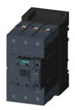
power contactor, AC-3 95 A, 45 kW / 400 V 1 NO + 1 NC, 110 V AC, 50 Hz Hz 120 V/60 Hz 3-pole, 3 NO, Size S3 screw terminal
