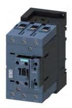
Contactor, AC-3, 55 kW/400 V 1 NO+1 NC, 110 V AC/50 Hz 120 V/60 Hz 3-pole, 3 NO, Size S3 Screw terminal
