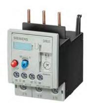
Overload relay 18...25 A For motor protection Size S2, Class 10 Contactor mounting Main circuit: Screw terminal Auxiliary circuit: Screw terminal Manual-Automatic-Reset !!! Phased-out product !!! Successor is SIRIUS 3RU2 Preferred successor type is >>3RU2136-4DB0<<
