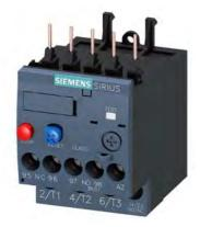
Overload relay 1.4...2.0 A Thermal For motor protection Size S00, Class 10 Contactor mounting Main circuit: Screw Auxiliary circuit: Screw Manual-Automatic-Reset
