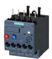
Overload relay 1.8...2.5 A Thermal For motor protection Size S00, Class 10 Contactor mounting Main circuit: Screw Auxiliary circuit: Screw Manual-Automatic-Reset
