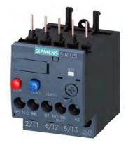
Overload relay 3.5...5.0 A Thermal For motor protection Size S00, Class 10 Contactor mounting Main circuit: Screw Auxiliary circuit: Screw Manual-Automatic-Reset
