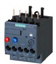
Overload relay 11...16 A Thermal For motor protection Size S00, Class 10 Contactor mounting Main circuit: Screw Auxiliary circuit: Screw Manual-Automatic-Reset
