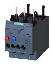
Overload relay 20...25 A Thermal For motor protection Size S0, Class 10 Contactor mounting Main circuit: Screw Auxiliary circuit: Screw Manual-Automatic-Reset
