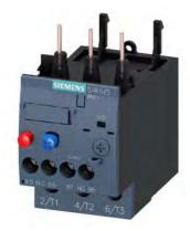
Overload relay 34...40 A Thermal For motor protection Size S0, Class 10 Contactor mounting Main circuit: Screw Auxiliary circuit: Screw Manual-Automatic-Reset
