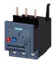
Overload relay 70...80 A Thermal For motor protection Size S2, Class 10A Contactor mounting Main circuit: Screw Auxiliary circuit: spring-type terminal Manual-Automatic-Reset
