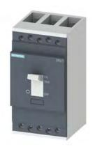
Molded case circuit breaker 3RV1 for motor protection Standard switching capacity Rated current In = 160 A electronic release Short-circuit protection adjustable 6-13 x In Overload protection adjustable 0.4-1 x In, Class 10A-31 Icu = 120 kA at 400 V 3-pole, Screw terminal including phase barriers
