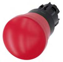
EMERGENCY STOP mushroom pushbutton, 22 mm, round, plastic, red, 40 mm, positive latching, acc. to EN ISO 13850, pull-to-unlatch mechanism
