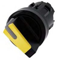
Selector switch, illuminable, 22 mm, round, plastic, yellow, selector switch, short, 2 switch positions O-I, latching, actuating angle  $90^\circ$ , 10:30h/13:30h
