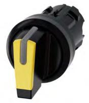
Selector switch, illuminable, 22 mm, round, plastic, yellow, selector switch, short, 3 switch positions I-O-II, latching, actuating angle  $2x45^{\circ}$ , 10:30h/12h/13:30h
