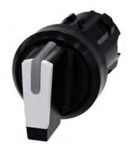
Selector switch, illuminable, 22 mm, round, plastic, white, selector switch, short, 3 switch positions I>O<II, momentary contact type, actuating angle  $2x45^{\circ}$ , 10:30h/12h/13:30h
