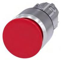
Mushroom pushbutton, 22 mm, round, metal, shiny, red, 30 mm, latching, Pull-to-unlatch mechanism
