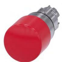
EMERGENCY STOP mushroom pushbutton, 22 mm, round, metal, shiny, red, 30 mm, positive latching, acc. to EN ISO 13850, rotate-to-unlatch
