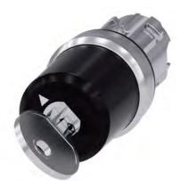
key-operated switch Siemens, 22 mm, round, metal, shiny, lock number SSG10, with 2 keys, 2 switch positions O-I, latching, actuating angle 90°, 10:30h/13:30h, key removal O
