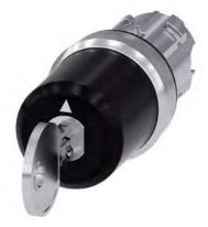
key-operated switch Siemens, 22 mm, round, metal, shiny, lock number SSG10, with 2 keys, 3 switch positions I>O<II, momentary contact type, actuating angle  $2x45^{\circ}$ , 10:30h/12h/13:30h, key removal O
