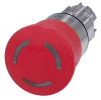
EMERGENCY STOP mushroom pushbutton, illuminable, 22 mm, round, metal, shiny, red, 40 mm, positive latching, acc. to EN ISO 13850, rotate-to-unlatch
