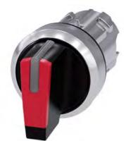
Selector switch, illuminable, 22 mm, round, metal, shiny, red, selector switch, short, 3 switch positions I-O-II, latching, actuating angle 2x45°, 10:30h/12h/13:30h
