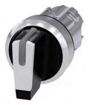
Selector switch, illuminable, 22 mm, round, metal, shiny, white, selector switch, short, 3 switch positions I>O<II, momentary contact type, actuating angle  $2x45^\circ$ , 10:30h/12h/13:30h
