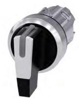
Selector switch, illuminable, 22 mm, round, metal, shiny, white, selector switch, long, 3 switch positions I-O-II, latching, actuating angle  $2x45^{\circ}$ , 10:30h/12h/13:30h
