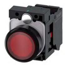
Illuminated pushbutton, 22 mm, round, plastic, red, pushbutton, flat, momentary contact type, with holder, 1 NC, LED module with integrated LED 24 V AC/DC, Spring-type terminal
